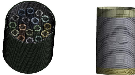
Figure 3. Mesh of the transverse magnetic field heat treatment furnace. Copyright: Drawn with Ansys Workbench 2022 R1.
