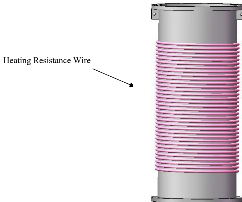
Figure 8. Model of a heating resistance wire with an optimized winding pattern. Copyright: Drawn with SolidWorks 2022.
