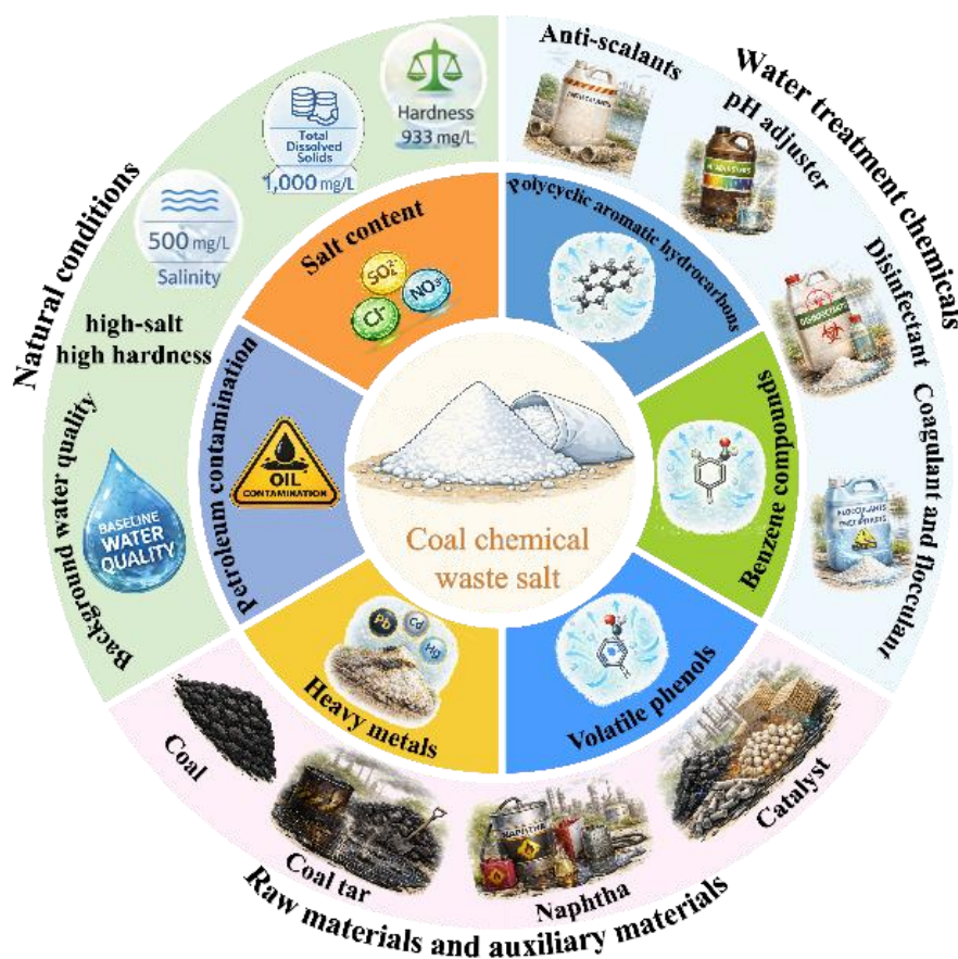
Figure. 1 Analysis of the composition and sources of waste salt from coal chemical processing. Created by the authors using Microsoft PowerPoint 2024.
